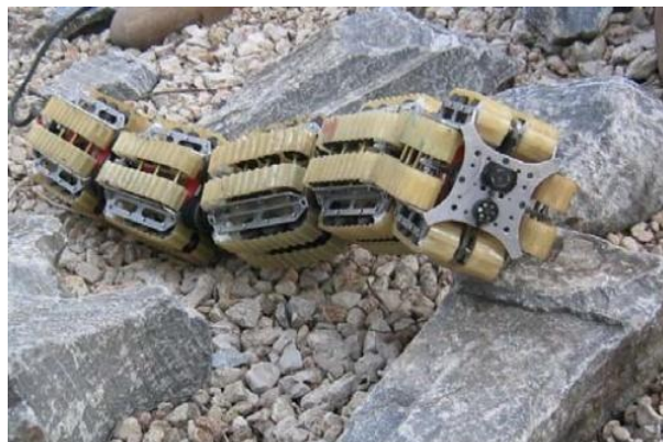
Figure 16: Snake-Inspired Robot “OmniTread OT-8” (Courtesy of Johann Borenstein, University of Michigan) [23].
