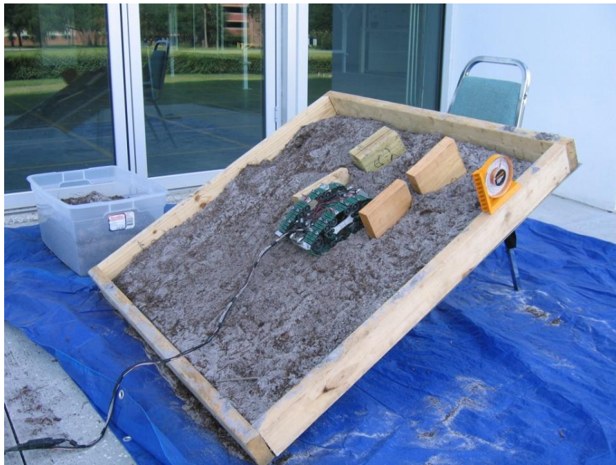
Figure 29: Robot Testing in Sandbox on a 30 Degree Slope.
