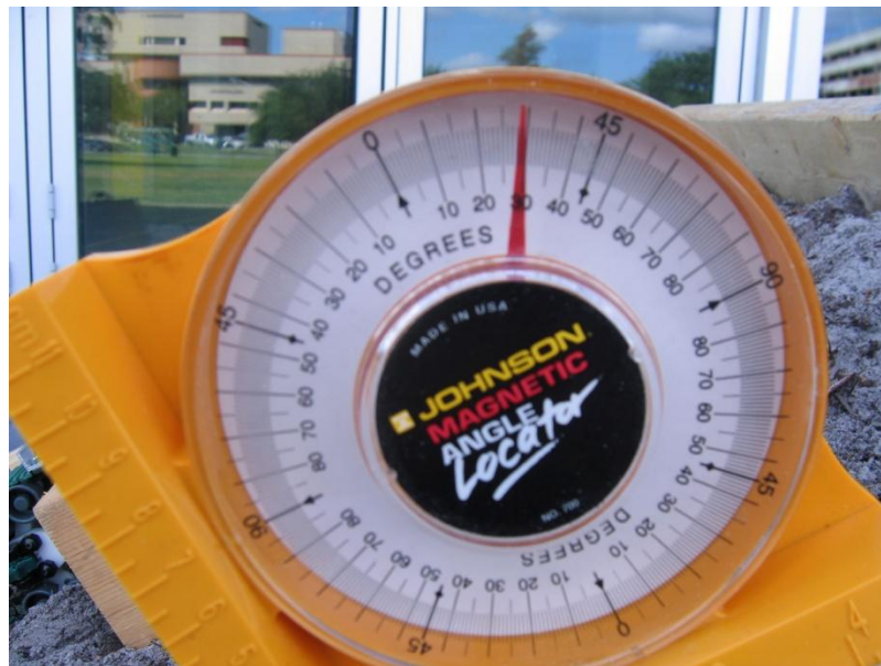
Figure 30: Inclinometer on the Sandbox Set at 30 Degrees.
