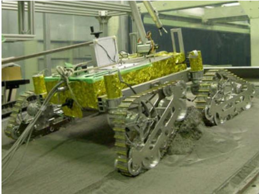
Figure 25: Rocker Suspension Displayed on Lunar Tracked Vehicle [21].
